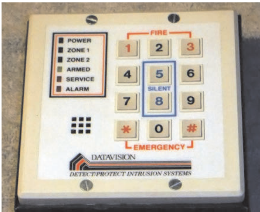
■ FIGURE 5. The completed keypad interface.
